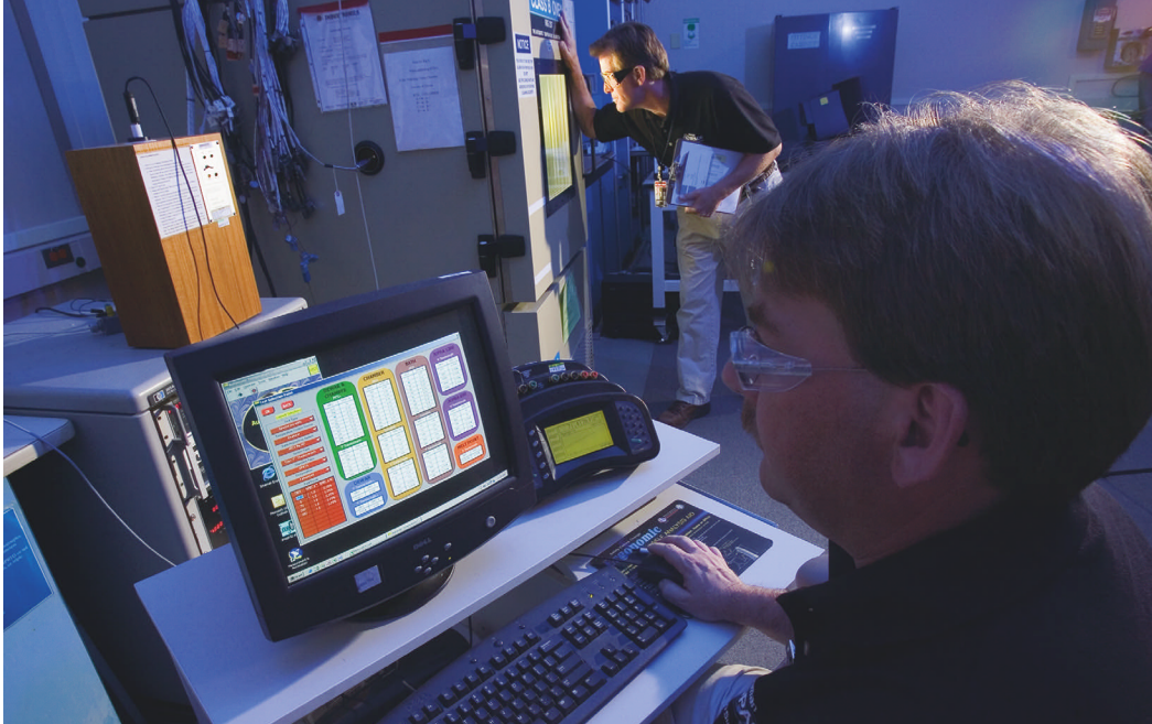
Engineer for methods and standards Scott Shepard (back) develops calibration procedures and provides technical assistance to the metrology lab. Technician Dave Zisk (foreground) calibrates and certifies instrumentation used for production testing of environmental controls.
